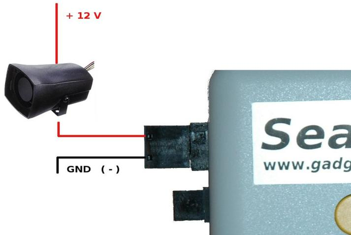
The terminal “-“ has to be connected to GND ( battery -12 Volt )
